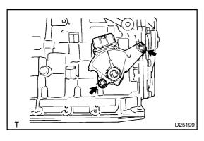
(e) Align the groove with neutral basic line, tighten the 2 bolts. **Torque: 5.4 N·m (55 kgf·cm, 48 in.·lbf)**
