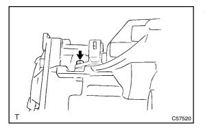
(c) Install the transmission wire and bolt. Torque: 5.4 N·m (55 kgf·cm, 48 in.·lbf)
