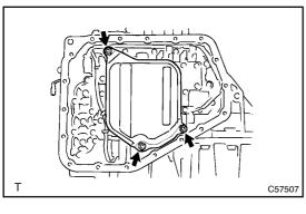
(b) Install the oil strainer to the transaxle assy with 3 bolts. **Torque: 9.8 N·m (100 kgf·cm, 7 ft·lbf)**
