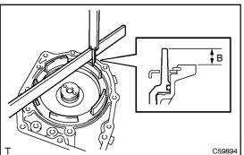
(b) As shown in the illustration, place a straight edge on the O/D brake piston and measure the distance between the transaxle rear cover and straight edge using vernier calipers. (Dimension B)
