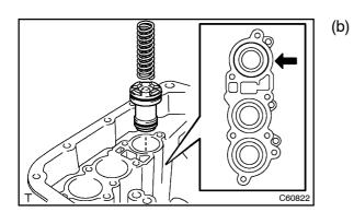
Install the  $B_1$  accumulator piston to the transaxle case.
