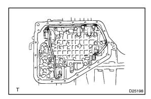
(c) Install the oil temperature sensor and solenoid connectors.
