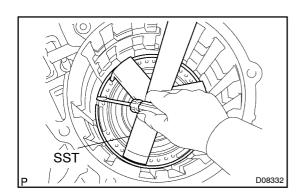
(b) Using SST, a press and a screwdriver, install the snap ring.
