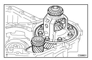
132. INSTALL DIFFERENTIAL GEAR ASSEMBLY
