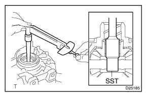
(b) Using SST and small torque wrench, measure the preload of the differential gear. SST 09564–32011
