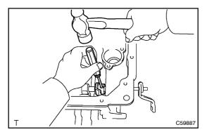
(b) Using a pin punch and hammer, drive out the pin.(c) Remove the manual valve lever shaft and manual valve lever.
