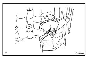
(f) Using a screwdriver, stake the nut with the lock washer.
