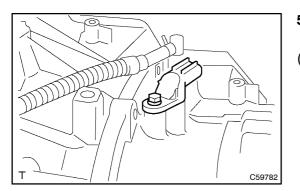
(b) Remove the 2 bolts, and pull out the neutral start switch.
