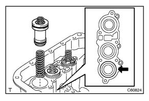
(b) Coat the piston with ATF and install it to the transaxle case.
