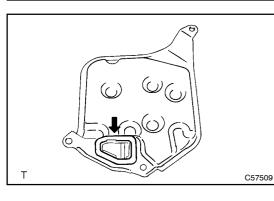
(b) Remove the gasket from the oil strainer.
