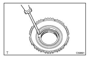
(b) Using a screwdriver, remove the one way clutch hole snap ring and remove the 1 way clutch No. 1 from the 2nd brake hub.
