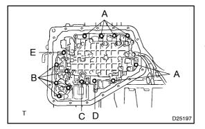
(b) Torque the 14 bolts at the same torque each.
