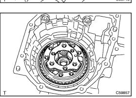
(c) Using a chisel and a hammer, stake the counter drive gear nut.
