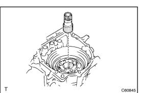
56. REMOVE PLANETARY SUN GEAR SUB-ASSY
