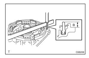
(b) As shown in the illustration, place a straight edge on the O/D brake piston and measure the distance between the transaxle rear cove and straight edge using vernier calipers. (Dimension B)
