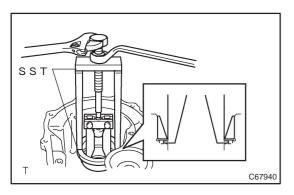
(b) Using SST, remove the front differential case RH tapered roller bearing outer race from the transaxle housing. SST 09387–00040 (09387–02020, 09387–02010)
