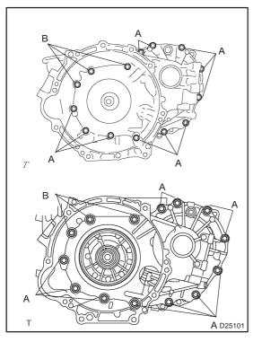
(b) Install the 14 bolts and transaxle housing.
