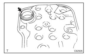
(b) Remove the O-ring from the oil stainer.
