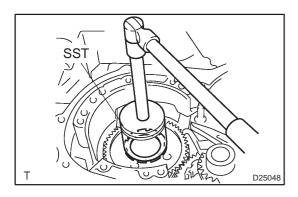
(c) Using SST, remove the nut and lock washer. SST 09387–00120
