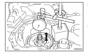
(b) Using a dial indicator, measure the rickety of intermediate shaft.
