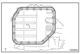
(b) Install the oil pan sub–assy and 19 bolts.
