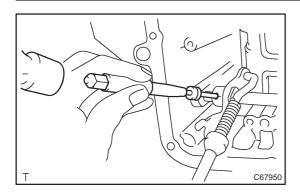
(c) Using a pin punch and hammer, drive in the pin.
