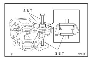
(b) Using SST and a press, install the shim and bearing outer race to the transaxle case.
