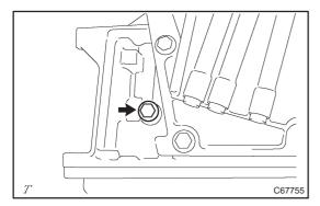
(c) Install the screw plug.
