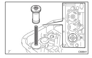
(b) Install the spring and  $B_2$  accumulator piston.
