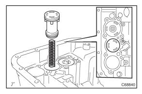
(b) Install the spring and  $C_3$  accumulator piston.
