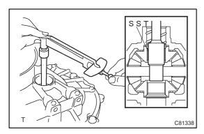
(c) Using SST and small torque wrench, measure the preload of the differential gear.
