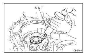
(d) Using SST and a hammer, stake the lock nut washer. SST 09930–00010
