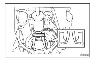
(c) Using SST, remove the counter drive gear bearing rear outer race from the transaxle case. SST 09308–00010
