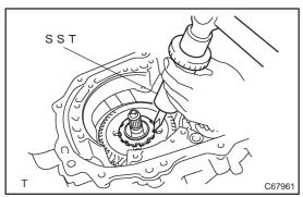
(b) Using SST and a hammer, unstake the lock washer. SST 09930–00010
