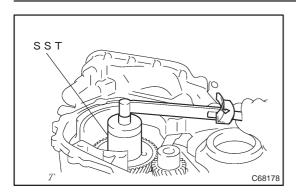
(b) Using SST, install a new lock washer and nut. SST 09387–00120
