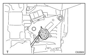
(h) Using a screwdriver, stake the nut with the lock washer.
