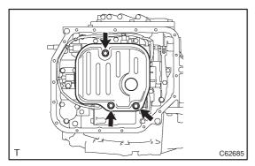
(b) Install the oil strainer and 3 bolts.
