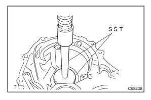
(b) Using SST and a press, install the tapered roller bearing to the transaxle housing.
