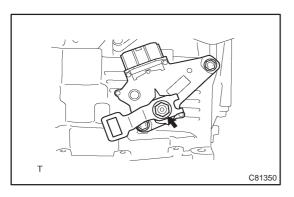
(i) Install the control lever, washer and nut.
