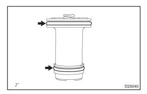
(b) Remove the 2 O–rings from the C<sub>2</sub> accumulator piston.
