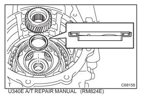
Install the planetary sun gear and needle roller bearing to (a) the planetary gear assy.
