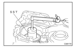
(c) Using SST and a small torque wrench, while turning to counter drive gear 60 turn par minute and measure the rotating torque.
