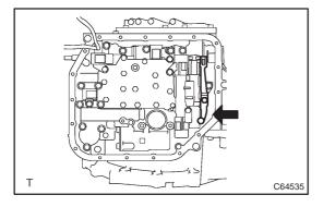
(c) Remove the 2 bolts, detente spring cover and detente spring.
