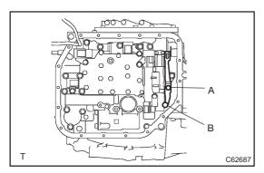
(b) Install the detente spring, detente spring cover and 2 bolts.
