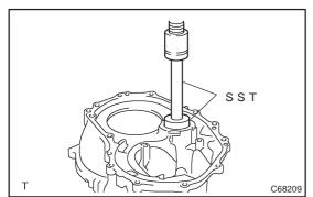
(b) Using SST and a press, install the cylindrical roller bearing to the transaxle housing.
