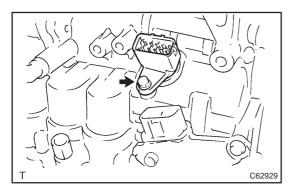
(c) Install the bolt and transaxle wire.
